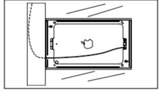
Connect the iPad and place it in the bezel. Attach the bezel to the bracket. Adhere the Surface Mount bracket to the glass close to the channel.
