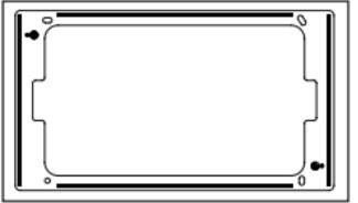
Adhere the adhesive strips on the back of the Surface Mount bracket as shown.
